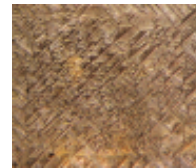
Fig. 3. Catalyst imprint on diamond's cubic face reveal remarkable alignment of lattices between solidifying catalyst metal and growing diamond crystal.
